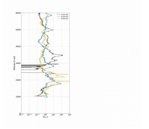
Figure 1: Gradient Richardson number computed from the radiosoundings
