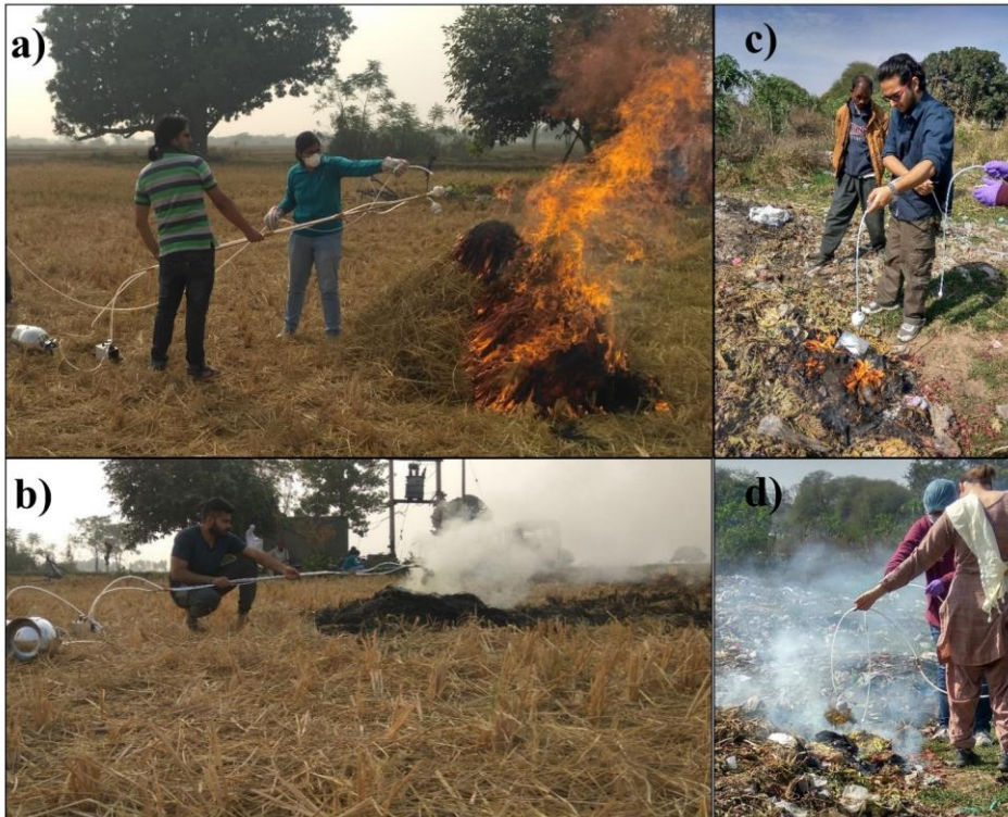
Figure S1: Whole air sample collection from a) paddy stubble fire: flaming; b) paddy stubble fire: smouldering; c) garbage fire: flaming; and d) garbage fire: smouldering. The flaming and smouldering fires were distinguished based upon the presence of flame and white smoke as per past experiences (Chandra et al 2017, Kumar et al., 2018).
