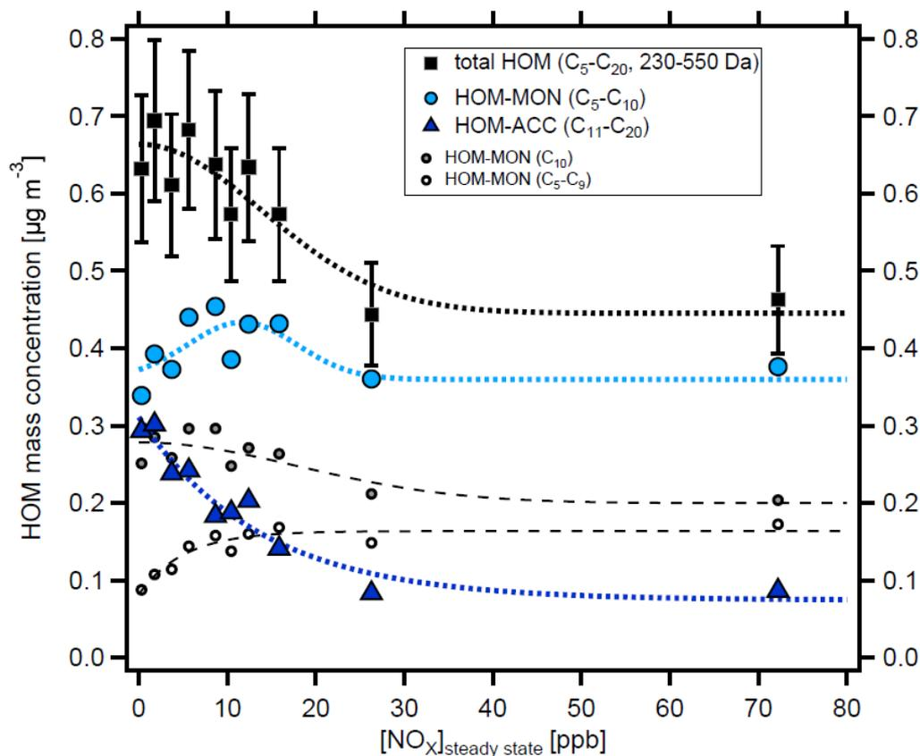
5 Figure 3. Mass concentration of HOM products in dependence on  $[\text{NO}_x]_{\text{ss}}$  in  $\alpha$ -pinene photo-oxidation experiments.  $\text{C}_5$ - $\text{C}_{20}$
