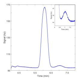
Figure 2. Sample chromatogram showing  $N_2O$  peak at a retention time of 6.1 minutes and  $SF_6$  peak at a retention time of 7.0 minutes. Upper-right corner inlay shows an enlarged plot of the  $SF_6$  peak.
