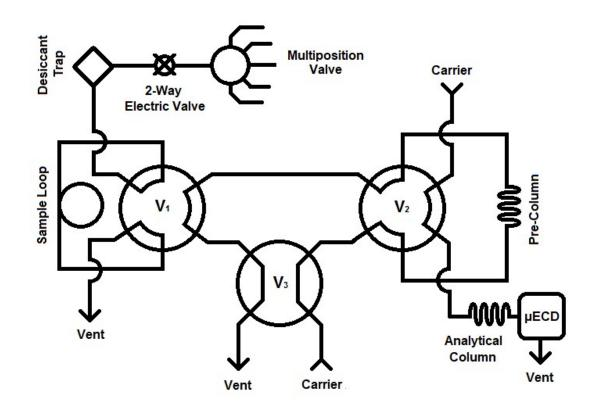
Figure 1. Schematic view of the analytical system for sample evaluation. The system is shown in "back-flush" mode.  $V_1 = Valve 1$ ,  $V_2 = Valve 2$ ,  $V_3 = Valve 3$ .
