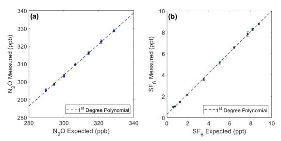
Figure 4. Measurement linearity from plots of measured mole fraction vs. expected mole fraction of  $N_2O$  (a) and  $SF_6$  (b). Expected mole fraction is calculated from the NOAA reference mole fraction (328.71 ppb  $N_2O$  and 8.76 ppt  $SF_6$ ) after dilution with ultra-pure air. Error bars represent 1 $\sigma$  total uncertainty.
