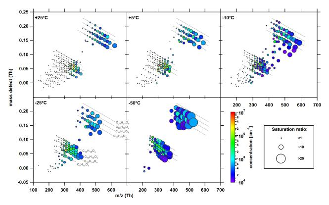
Figure 5: Composition of the measured gas-phase HOMs at different temperatures and their saturation ratio 1080 distribution.
