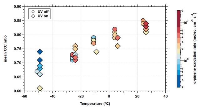
1030 Figure 2: Mean oxygen-to-carbon elemental ratio (O/C) of HOMs at different temperatures and various α-pinene oxidation rates.
