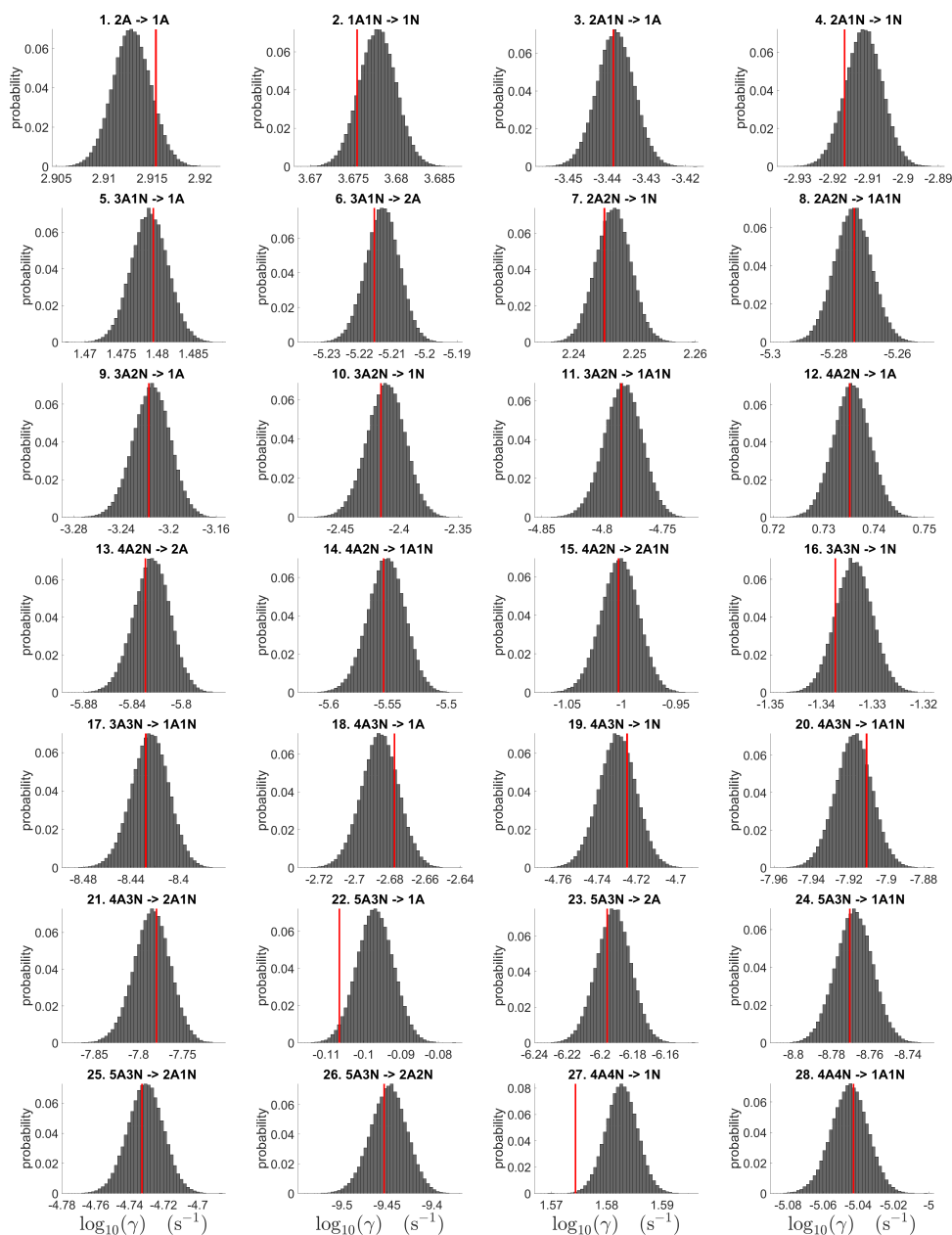
Figure D6. One-dimensional marginal distributions (for parameter indexes ranging from 1 to 28) of the base 10 logarithm of the evaporation rates (units given in \text{s}^{-1} ) at temperature 278 K obtained from a posterior distribution of thermodynamic parameters (cluster formation enthalpies and entropies) determined from steady-state cluster concentration measured at temperatures 278 K and 292 K. Red lines denote the baseline values from Ortega et al. (2012) used to generate the synthetic data. In reactions "A" stands for \text{H}_2\text{SO}_4 and "N" for \text{NH}_3 .
