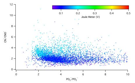
Bioaerosol (Aspergillus cellulase) particles ionized using different laser powers.
