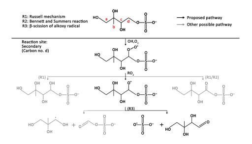
**Scheme 4.** Proposed reaction mechanism for the heterogeneous OH oxidation of potassium 3-methyltetrol sulfate ester at the carbon labelled d.
