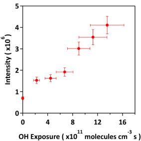
**Figure 2.** The evolution of the intensity of bisulfate ion (HSO<sub>4</sub><sup>-</sup>) as a function of OH exposure during the heterogeneous OH oxidation of potassium 3-methyltetrol sulfate ester at 70.8% RH.
