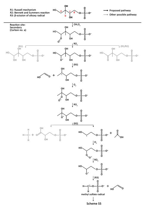
**Scheme 1.** Proposed reaction mechanisms for the heterogeneous OH oxidation of potassium 3-methyltetrol sulfate ester at the carbon labelled a.
