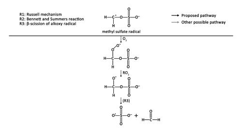
Scheme 5. Proposed reaction mechanism for the reactions of alkyl radical of methyl sulfate anion.
