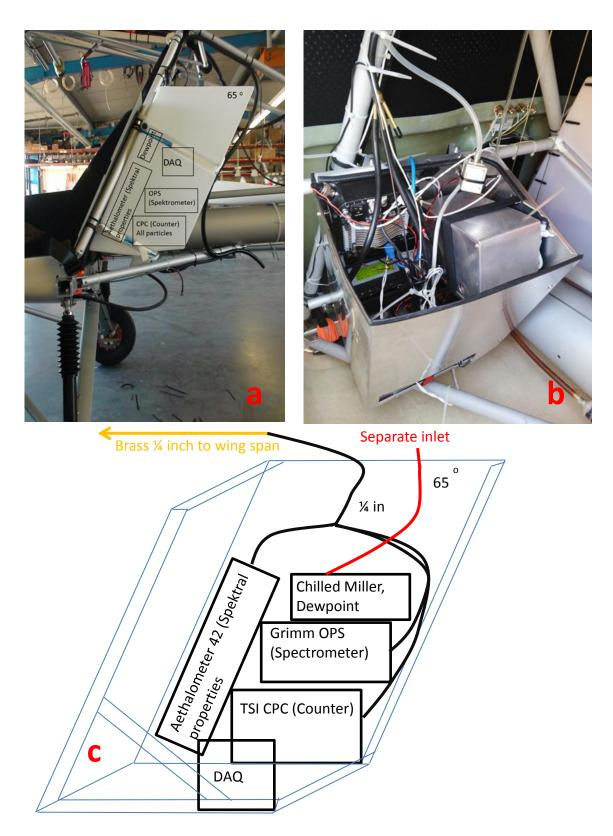
Figure S1: Testing and assembly of the instrument package inside IKARUS-C42 in the COMCO IKARUS station in Germany (a) field station in Pokhara Valley (b) sketch of the Instrument package (c)
