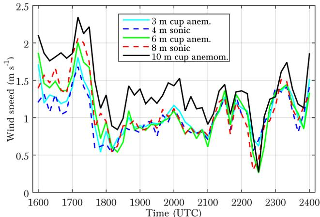
Figure IV: *Time series of the wind speed from 1600 to 2400 UTC on the 13/08/2017. Solid lines represent the measurements from cup anemometers, and dashed lines from sonic anemometers.*
