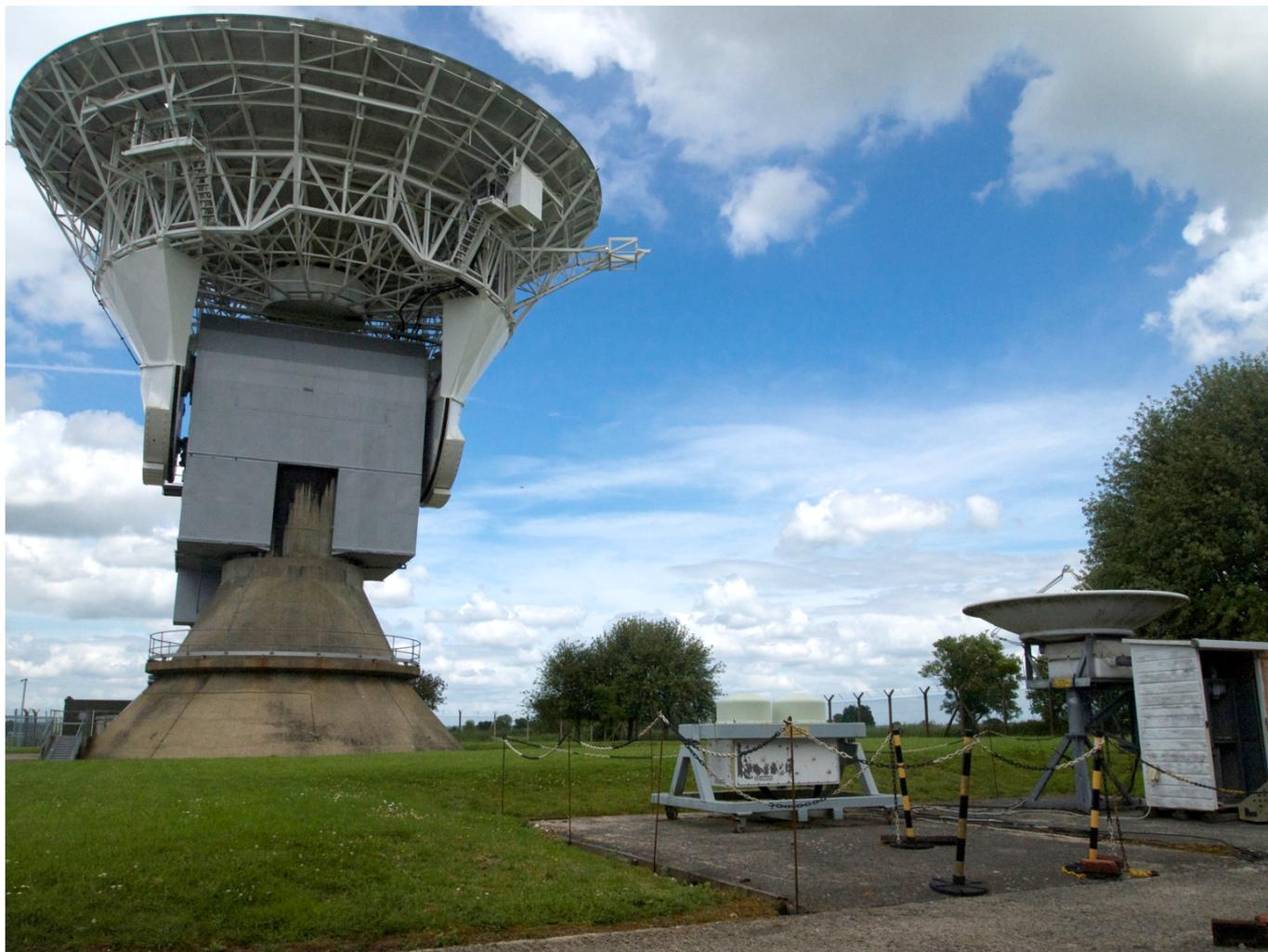
**Figure 1.** A photograph of the three co-located radars at the Chilbolton Observatory, Hampshire, England. From left to right: the 3-GHz CAMRa radar, 94-GHz radar and 35-GHz radar.
