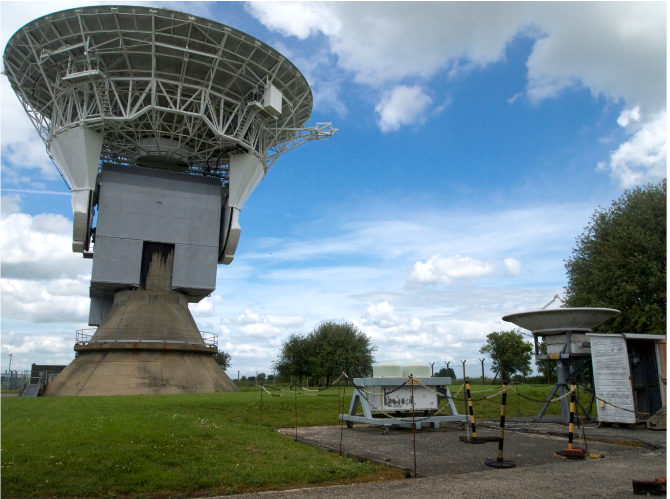
Figure 2. A photograph of the three co-located radars at the Chilbolton Observatory, Hampshire, England. From left to right: the 3-GHz CAMRa radar, 94-GHz radar and 35-GHz radar.
