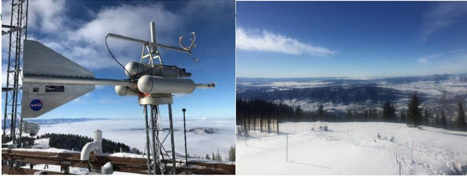
**Figure 1.** Recent picture of SPL probe stand with in and FSSP-100 in foreground, CIP in background, and sonic anemometer on top (left panel). View facing west over the railing (right panel).
