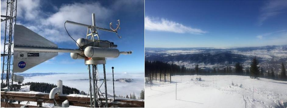
**Figure 1 (revised).** Recent picture of SPL probe stand used previously during StormVEx and IFRACS with FSSP-100 and sonic anemometer on top and DMT CIP and PIP (Precipitation Imaging Probe) on left and right sides, respectively. View facing west over the railing (right panel).
