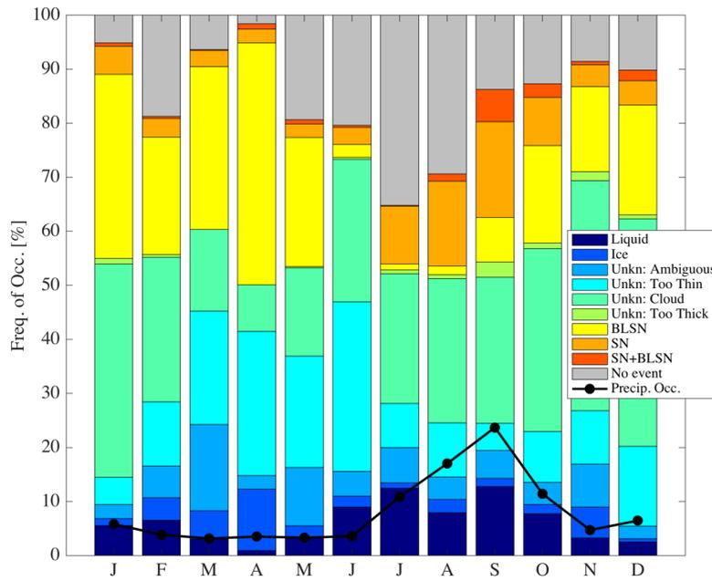
5 **Figure 5.** Composite monthly frequencies of occurrence of each classification. BLSN and SN refer to blowing snow and snow, respectively. Precipitation occurrence is the sum of SN and BLSN+SN.
