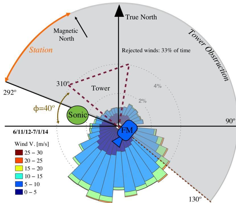
**Figure 1.** Schematic plan view of the field setup of the FM100 (blue icon labelled “FM”) on the tower (dashed triangle) at Summit Station. The green oval (“sonic”) is the position of the Metek sonic anemometer. The grey shaded area are the wind directions that were rejected and the orange arrow denotes the sector facing the station. The wind rose is also shown centered on the FM position.
