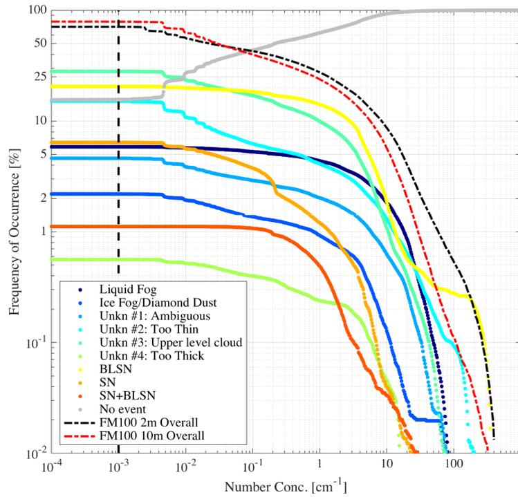
5 **Figure 3.** Percent of time clouds are identified in FM100 data at 2 m (black dashed) and 10 m (red dashed) as a function of threshold in number concentration. Colours show the same for the classifications that are reported in Figure 5.
