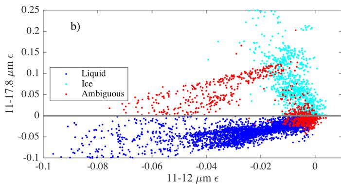
**Figure 4.** Example of phase classification using microwindow cloud emissivity measured by the AERI for the month of June.
