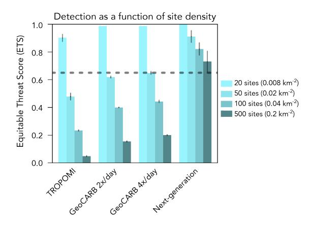
Figure 6. Equitable Threat Score (ETS) for each satellite observing configuration, varying the density of production sites
