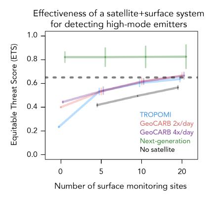
**Figure 8**: Effectiveness of a combined satellite and surface observing system for detecting high-mode emitters in an oil/gas field of 100 emitters over a 50×50 km<sup>2</sup> domain, as determined from joint inversion of the observations. The dashed line represents the ETS success criterion.
