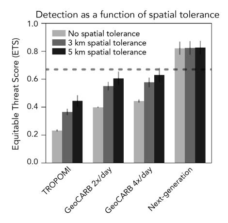
**Figure 7**: Effect of introducing spatial tolerance in the detection of high-mode emitters. Spatial tolerance is the radius within which a high-mode emitter must be located in order for a prediction to be called true positive (TP). The results are for an emission field with 100 production sites in the 50×50 km<sup>2</sup> domain. Only results from the L-1 inversion method are shown. The dashed line represents the ETS success criterion.
