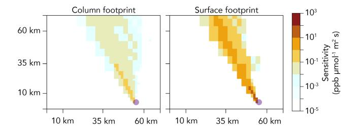
**Figure 3**: Sample sensitivities of observed atmospheric concentrations (column and surface) to surface emissions upwind, defining the emission footprint for that observation. Values are shown here for a particular observation point (purple dot) and time (October 19, 2013 at 09 LT). Concentrations are in mixing ratio units of ppb (dry column mean mixing ratio for the column) and emissions are in units of μmol m<sup>-2</sup> s<sup>-1</sup>.
