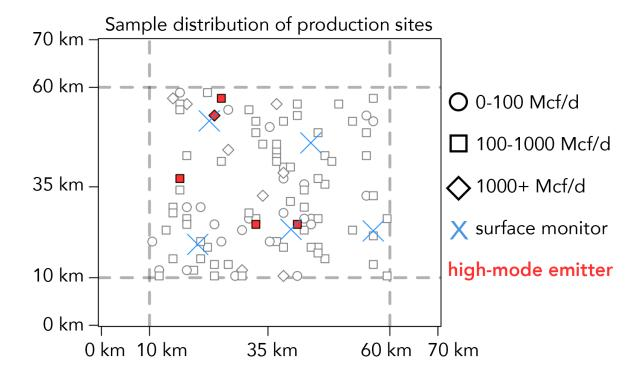
Figure 2. Sample realization of emissions from a hypothetical oil/gas production field with 100 production sites of different production size categories (symbols) within a 50×50 km² domain (dashed line). Different production size categories are shown with symbols. Red shading indicates high-mode emitters. Blue symbols mark the locations of five surface air monitoring sites placed according to the *k*-means algorithm.
