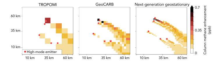
**Figure 4**: Simulated noiseless methane column enhancement for sampling by single overpasses of TROPOMI, GeoCARB, and a next-generation high-resolution geostationary satellite (Table 1). Emission field is that of Figure 2. The locations of the five high-mode emitters in that field are indicated. Values are for 22 October 2013 at 13 LT.
