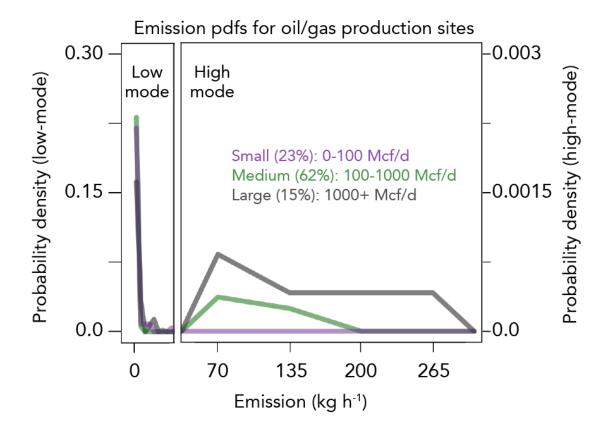
**Figure 1**. Probability density functions (pdfs) of emissions for oil/gas production sites of different production size categories (small, medium, and large), taken from Barnett Shale observations (Lan et al., 2015; Rella et al., 2015; Yacovitch et al., 2015). Note the difference in y-axis scales between the left (low-mode) and right (high-mode) panels. The axis break at 40 kg h<sup>-1</sup> represents the threshold for flagging an emitter as high.
