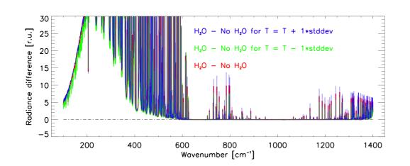
**Fig. 2.** Differences between downwelling radiances computed using an atmospheric profile with and without water vapour (in red), and for 2 cases of temperature perturbations (+/- 1 standard deviation, respecti
