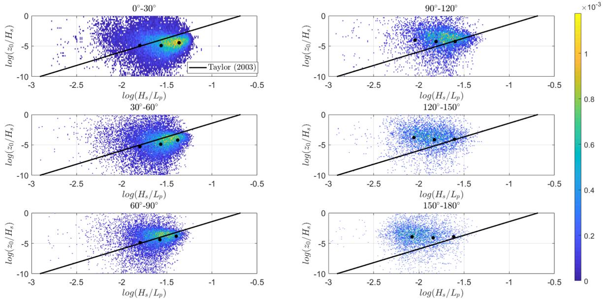
Figure R2: The dimensionless roughness is plotted against the wave steepness for 6 different groups of alignment for the ASIT measurement mast and for the FINO1 data sets combined. The solid black line represents the roughness parameterization proposed by Taylor and Yelland (2001). The color scale to the right indicates the probability of the occurrence (%) of the measurement points.
