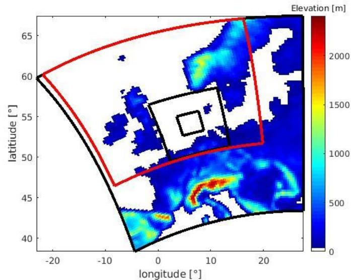
Figure R7: Domain set up for COAWST simulations centered around the FINO1 location. The black lines represent the atmospheric domains, which are three nested domains. The red lines represent the nested wave domains.
