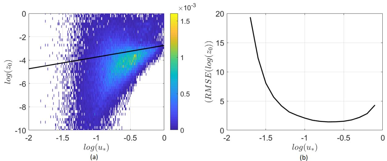
Figure R4: (a) The roughness is plotted against the friction velocity. The black line is the Charnock parameterization with  $\alpha = 0.018$ . The color scale to the right indicates the probability of occurrence (%) of the measurement point of both ASIT and FINO1 data sets. (b) The root mean square error of the measurement points compared to the Charnock parameterization.
