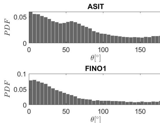
Figure R3: Probability density function (PDF) of the angle between the wind and wave direction for (up)the ASIT measurement mast and (down) for the FINO1 mast.
