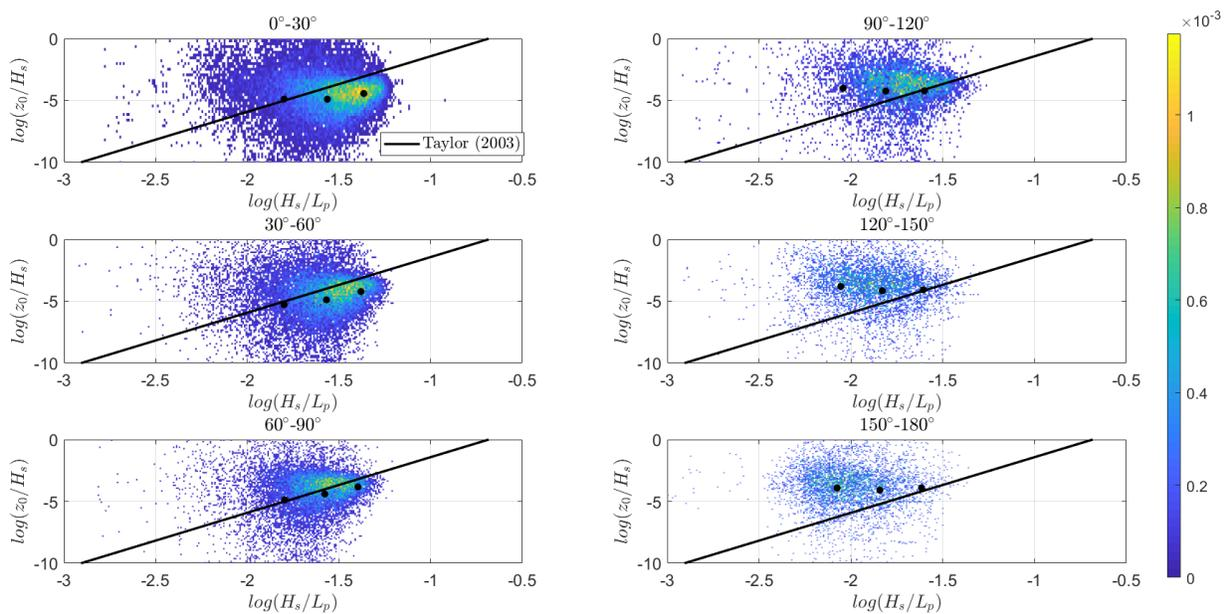
Figure R6: The dimensionless roughness is plotted against the wave steepness for 6 different groups of alignment for the ASIT measurement mast and for the FINO1 data sets combined. The solid black line represents the roughness parameterization proposed by Taylor and Yelland (2001). The color scale to the right indicates the probability of the occurrence (%) of the measurement points.
