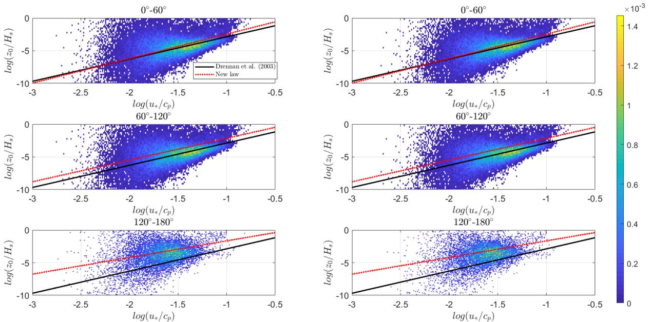
Figure R5: The dimensionless roughness is plotted against the inverse wave age parameter for 3 different groups of alignment for (left) measurements including upward momentum and (right) measurements excluding upward momentum. The solid black line
