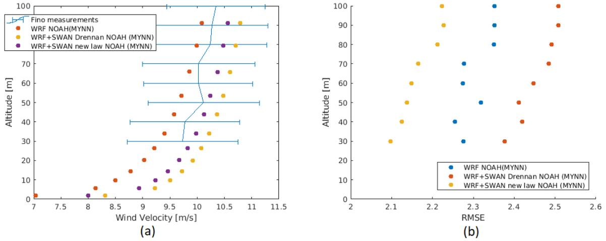
Figure R8: (a) Mean velocity profile of (1) the FINO1 measurements together with one standard deviation (2) the results of an atmospheric (WRF) only simulation (3) the results of a coupled atmospheric (WRF) wave (SWAN) model using Drennans roughness parameterization and (4) the results of a coupled atmospheric (WRF) wave (SWAN) model using the newly proposed roughness parameterization. (b) The RMSE from the simulation results compared to the FINO1 measurements for simulation (2), (3) and (4).
