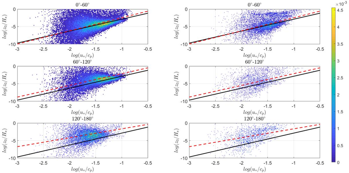
Figure R1: The dimensionless roughness length is plotted against the inverse wave age parameter for 3 different groups of alignment for (left) the ASIT measurement mast and (right) for the FINO1 data set. The solid black line represents the roughness parameterization proposed by Drennan et al. (2003), the dashed red line is the new proposed roughness parameterization. The color scale to the right indicates the probability of the occurrence (%) of the measurement points.
