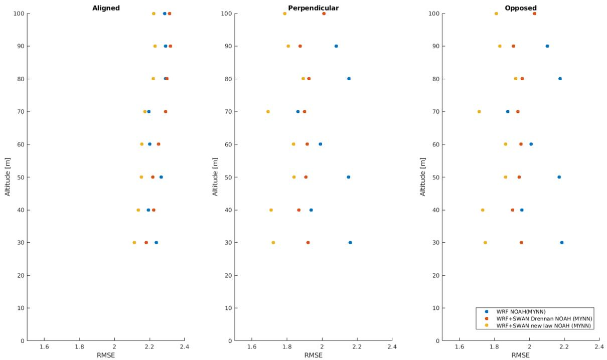
Figure R9: RMSE for three different classes of alignment (aligned 0°-60°, perpendicular 60°-120°, opposed 120-180°), for (1) the WRF only simulation (2) WRF+SWAN simulation with the roughness length parameterization of Drennan and (3) WRF+SWAN simulation with the newly proposed roughness length parameterization.
