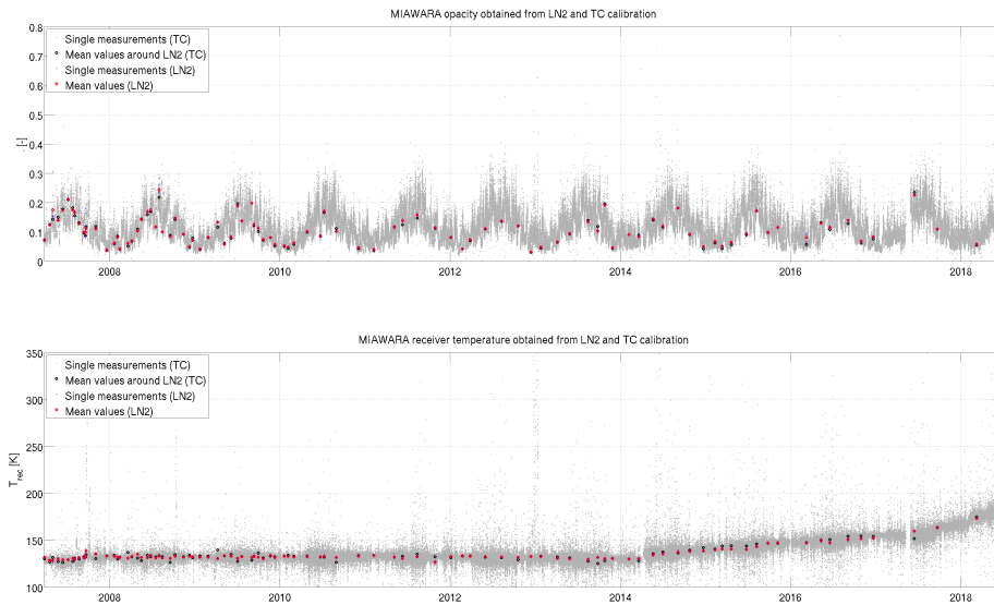
Figure 1. Development of the tropospheric opacities and the MIAWARA receiver temperatures as obtained from tipping curve (TC) (operational, grey dots) and regular liquid nitrogen (LN2) verification calibrations (mean values shown by red markers). The mean values around LN2 can be compared to the mean values around TC that are shown by the black markers. The time period between April 2007 and May 2018 is shown.
