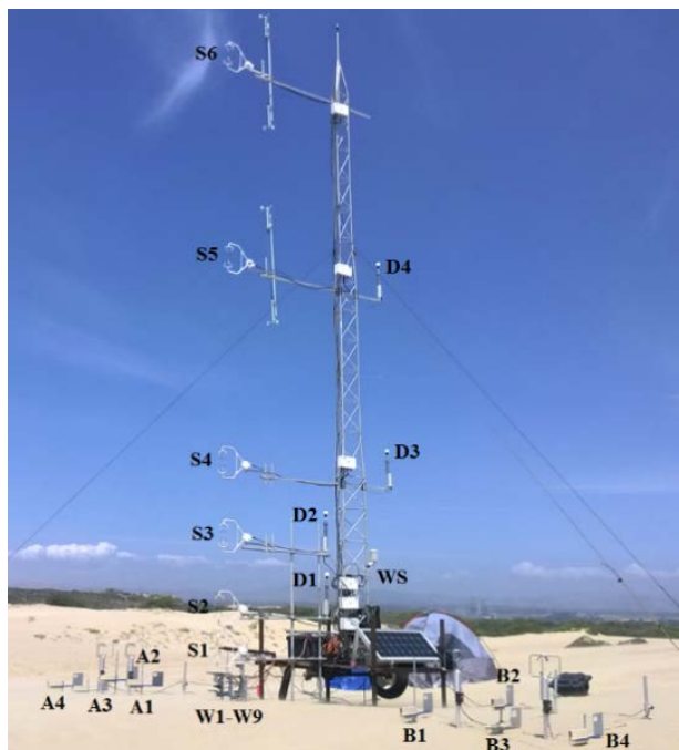
Figure 1: The experimental setup at Oceano Dunes. Instrumentation includes six sonic anemometers (S1-S6), nine Wenglor particle counters (W1-W9), eight Big Spring Number Eight sand samplers (A1-A4, B1-B4), four optical particle counters (D1-D4), and a weather station with temperature and humidity sensors (WS) (after Martin and Kok, 2017).
