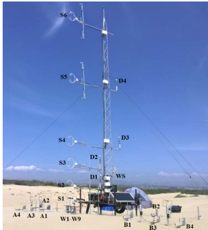
Figure 1: The experimental setup at Oceano Dunes. Instrumentation includes six sonic anemometers (S1-S6), nine Wenglor particle counters (W1-W9), eight Big Spring Number Eight sand samplers (A1-A4, B1-B4), four optical particle counters (D1-D4), and a weather station with temperature and humidity sensors (WS) (after Martin and Kok, 2017).
