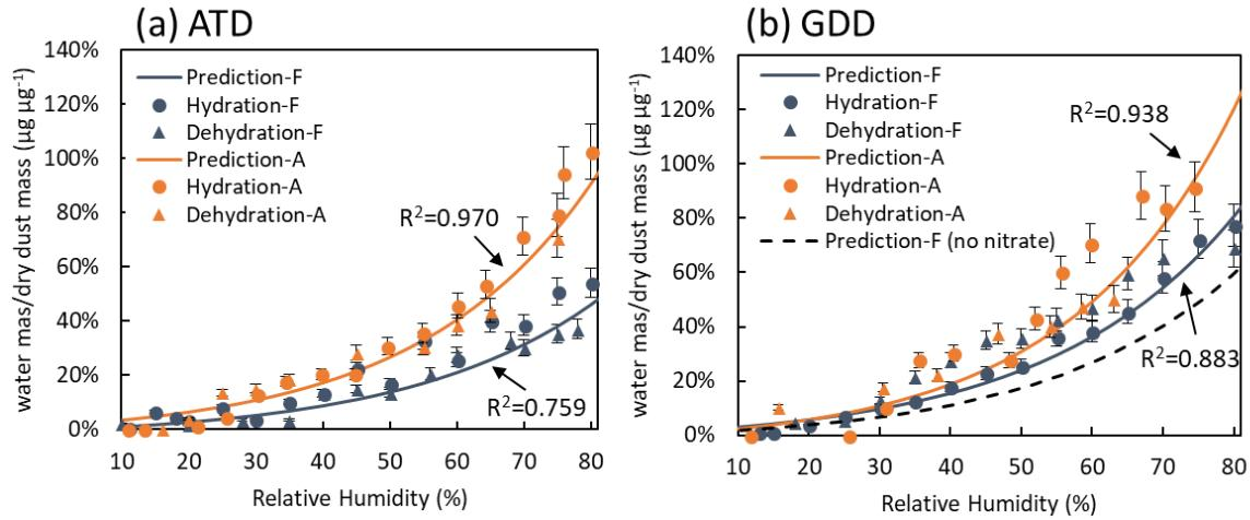
Figure 2. The fraction of water mass relative to the dry dust mass for fresh and photochemically aged (a) ATD and (b) GDD particles as a function of the relative humidity from 10% to 85%. “F” and “A” represent the fresh and aged dust particles, respectively. The water content for fresh GDD
