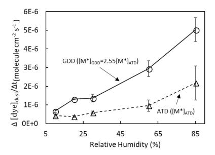
Figure 3. The dye degradation rate in the presence of ATD or GDD particles measured using a UV flow chamber under RH levels ranging from 10% to 85%. As a control, the photodegradation of malachite green in the absence of dust was measured, but the degradation was negligible. The error bars represent the standard deviations.
