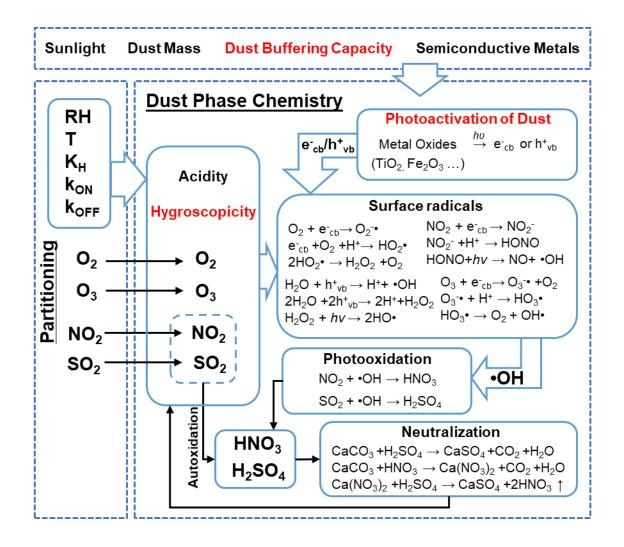
Figure 1. The overall schematic of dust phase chemistry in the AMAR model.
