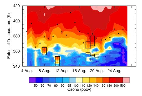
**Figure 1.** Daily variations of ozone mixing ratios (OMR) between 340 K and 430 K during 4-27 August 2013 from balloon measurements launched in Lhasa. The black dots represent the lapse rate tropopause. High tropospheric ozone is shown by the black rectangle.
