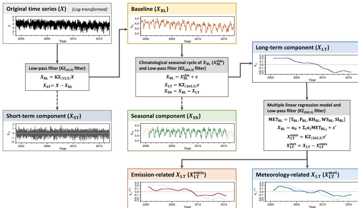
**Figure 2:** Schematic flowchart of temporal decomposition of air pollution time series (PM<sub>10</sub> in Seoul) into short-term, seasonal, and emission-related and meteorology-related long-term components.
