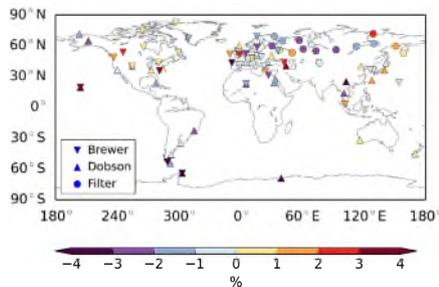
**Figure 1.** Mean total column ozone differences (%) between OMI-TOMS and Brewer, Dobson, and filter ozonometer measurements over July-August 2014. The colours blue to purple denote negative differences and the colours yellow to red refer to positive differences.
