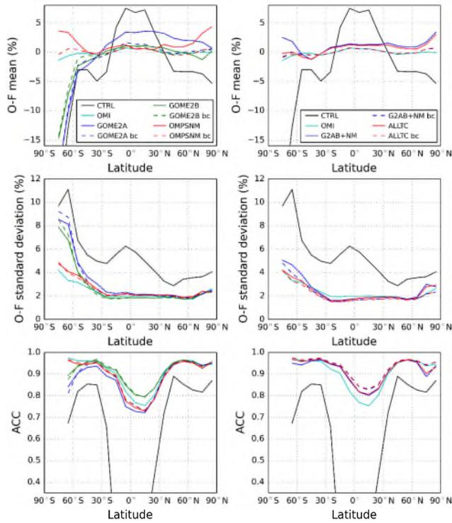
**Figure 8.** Zonal mean total column ozone statistics of mean differences (%), standard deviations (%), and anomaly correlation coefficients (ACC; unitless) as a function of latitude (degrees) for the comparison between OMI-TOMS measurements and short-term forecasts for July-August 2014. The legends in the top plots indicate the assimilation runs (see Table 6 for description) and apply to all plots in the same column.
