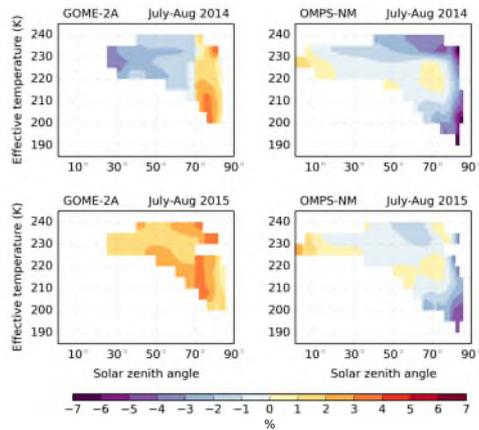
**Figure 7.** Mean total column ozone differences (%) between GOME-2A, OMPS-NM and collocated OMI-TOMS data as a function of ozone effective temperature (degrees Kelvin) and solar zenith angle (degrees) for the periods of July-August 2014 and July-August 2015. The colours blue to purple denote negative differences and the colours yellow to red refer to positive differences.
