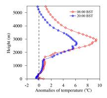
**Fig. 3.** Fig. S3 Vertical profiles of temperature anomalies at Wenjiang station (30.75 $^{\circ}$  N, 103.875 $^{\circ}$  E) measured by radiosonde (the averaged temperature during periods of deteriorating air quality in the eight
