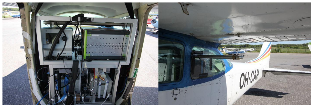
505 Figure 1. Instrumentation rack was installed inside the cabin (on the left) and the sample air for the 506 instrumentation was taken from a steel tube at 50 cm distance from the fuselage of the plane (on the 507 right).
