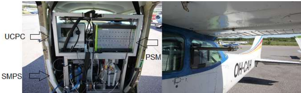
541 Figure 1. Instrumentation rack was installed inside the cabin (on the left) and the sample air for the 542 instrumentation was taken from a steel tube at 50 cm distance from the fuselage of the plane (on the 543 right). The main instruments (ultrafine-CPC, PSM and SMPS) are shown in figure.
