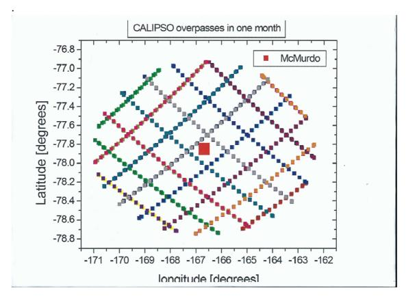
McMurdo. While CALIOP provides a resolution of 5 km (when integration is required due to low signal-to-noise ratio up to 135 km!) the air mass sampled by the ground-based lidar extends to at most 100 m. (30 km \* 3 mrad field of view of the telescope).
