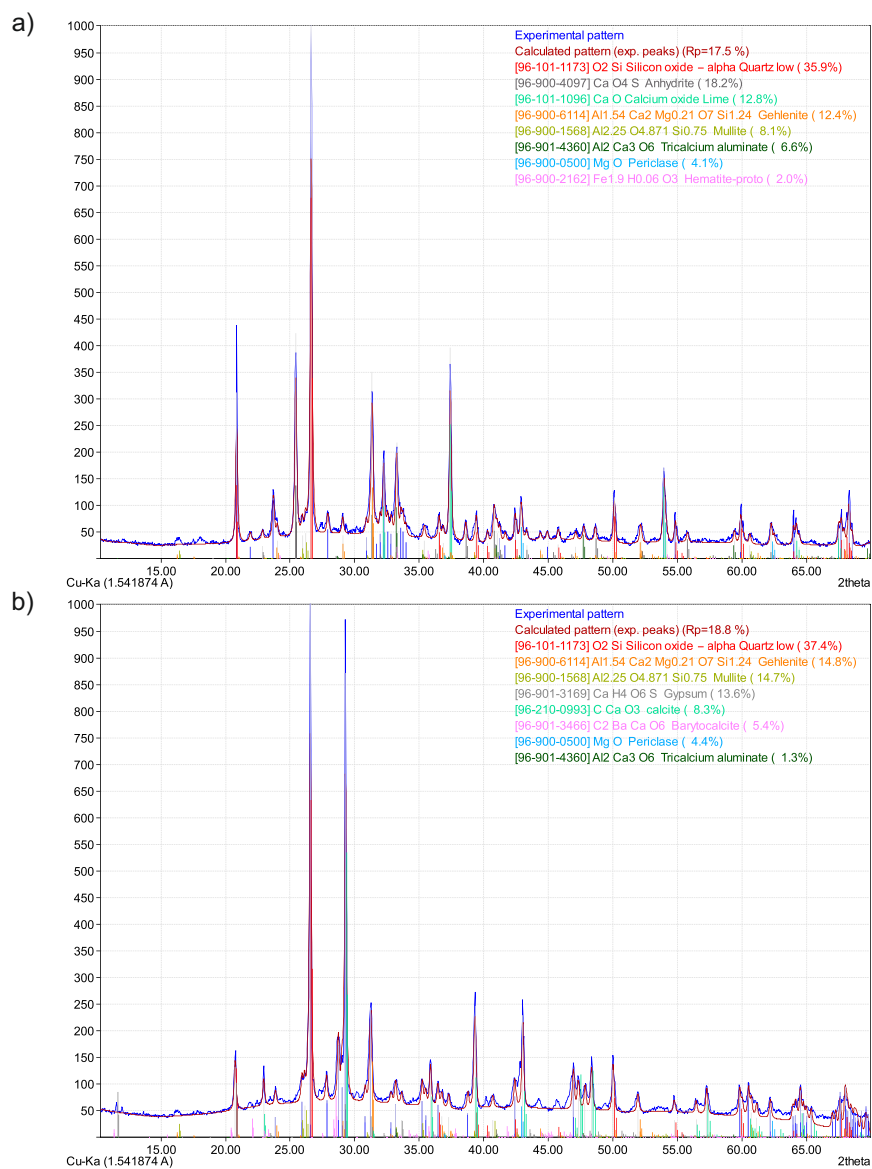
Figure S6. XRD patterns of a) dry bulk CFA1 and b) CFA1 after suspension and evaporation.
