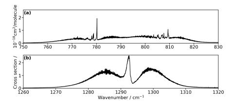
Figure 5. Example of an absorption cross section of ClONO<sub>2</sub> (a)  $\nu_4$ ,  $\nu_3$  and (b)  $\nu_2$  bands, measured by Wagner and Birk (2003) in a cuvette at a temperature of 297.4 K and pressure of 100 hPa.
