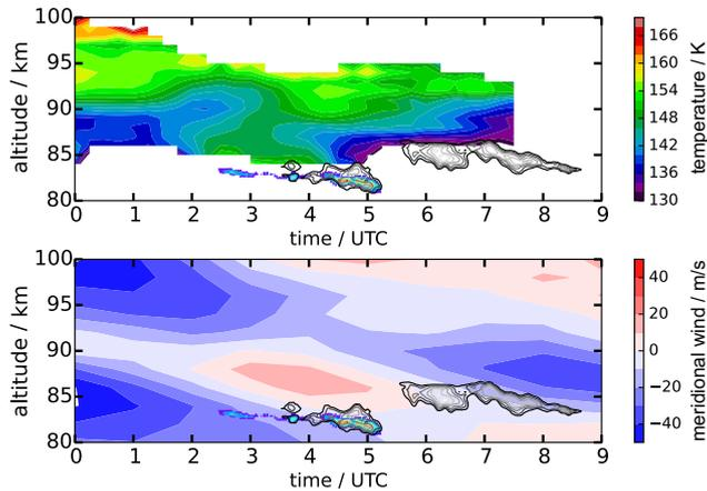
**Figure 6.** Temperature (top) and meridional wind (bottom) above Kühlungsborn during 26/27 June 2011. The MSE data is embedded in both panels for illustration as open grey contours and the NLC data in colored filled contours. Cloud 1: 2:30–5:15 UTC, Cloud 2: 5:30–8:40 UTC
