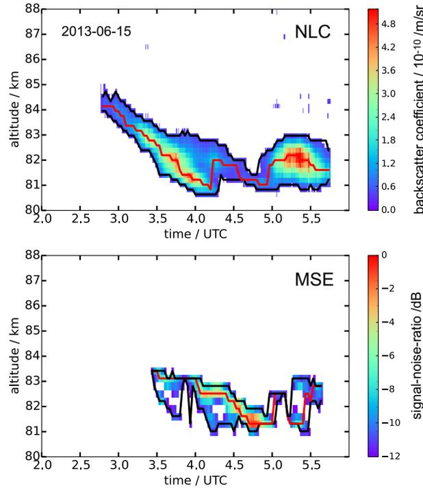
**Figure 1.** Examples for detection of NLC (top) and MSE (bottom) using observations on 15 June 2013. The black lines show the upper and lower edges ( $z_{low}^{low}$  and  $z_{up}^{up}$ ), the red line the layer maxima ( $z_{max}^{max}$ ). Edge detection is done on the temporal resolution of the radar (2 min). Edges are defined at  $\beta = 0.3$  (NLC) and  $SNR = -12$  dB (MSE).
