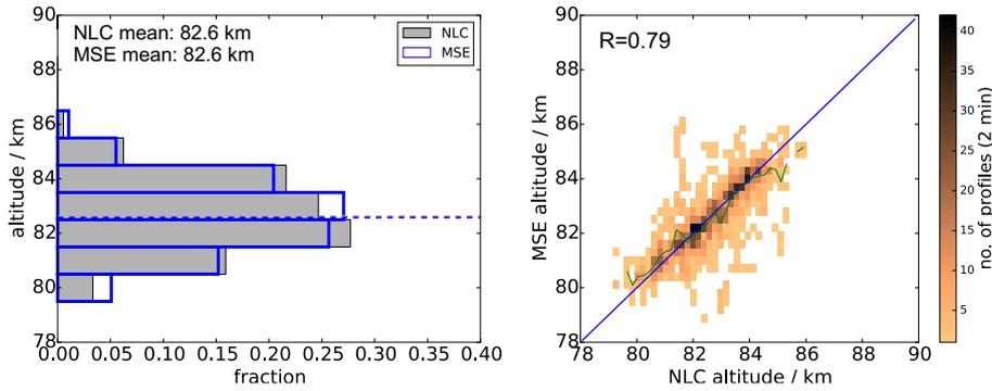
**Figure 3.** Comparison of lower edges of NLC and MSE ( $z_{NLC}^{low}$  and  $z_{MSE}^{low}$ ). a) Histogram with NLC edges in grey (filled) and MSE edges in blue (open histogram). Mean values are indicated by the dashed lines. b) Scatter plot of MSE and NLC edges. Only simultaneous soundings based on a 2 minute temporal resolution are evaluated. The green line in b) shows the average MSE lower edge altitude for each NLC edge bin and the blue line indicates identical altitudes.
