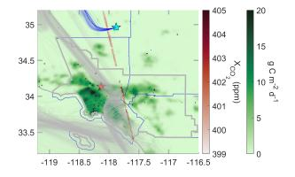
Figure 5. A visualization of OCO-2 observations and the forward model used in the flux inversion on June 20, 2015. The nadir track is shown starting at the bottom and  $\sim 117.6^{\circ}$ W and going towards the northwest. Observations are overlaid on the ODIAC prior at 14:00 (UTC-7). For every 5th sounding the set of backtrajectories is shown.
