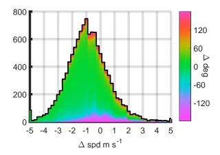
**Figure B1.** Histogram of Wind speed errors (HYSPLIT-measured) compared to surface observations at the San Gabriel airport. The mean error is  $-0.9 \text{ m s}^{-1}$  (-30 %), the 95 % confidence interval is [-3.7, 2.3] m s<sup>-1</sup>. The mean direction error is less than 5°, and 75 % of direction errors are within  $\pm 45^{\circ}$ .
