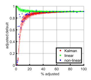
**Figure D1.** Effects of scaling a random subset of model data compared to no scaling. When fewer points are scaled, they are scaled by a larger amount. The Kalman filter and non-linear inversion are more affect by a few strong outliers than the linear inversion.
