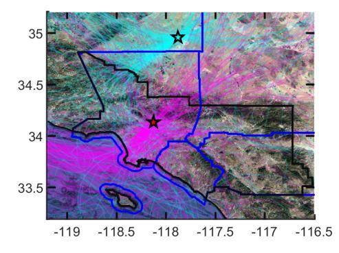
**Figure 2.** HYSPLIT 400 m a.g.l. back trajectories for NAM 12 km for 2015. For each day trajectories are shown ending at the 2 different TCCON receptor sites at 14:00 (UTC-7). Magenta trajectories end at Caltech. Cyan trajectories end at AFRC.
