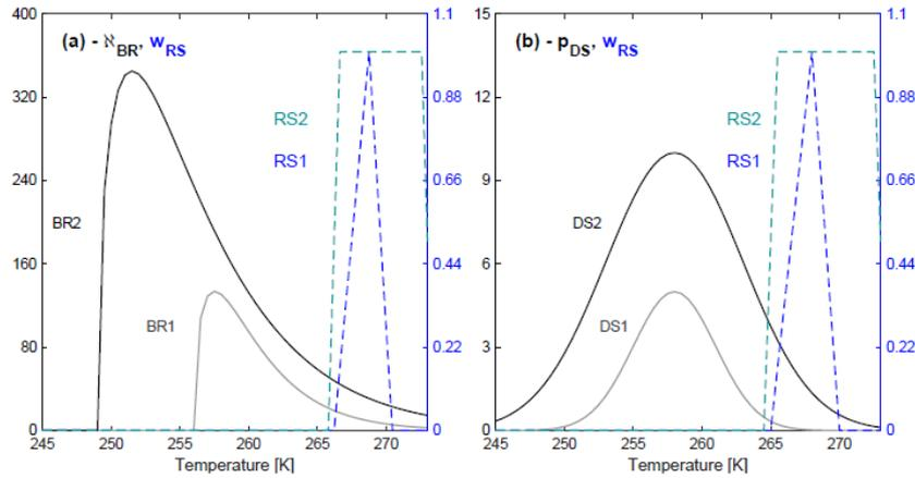
Figure 2 Fragment numbers, weightings, and probabilities from the secondary ice production parameterizations. In panel a, we show  $N_{BR}$  from both ice-ice collisional breakup simulations (BR1 and BR2) as well as the triangular and uniform  $w_{RS}(T)$ . In panel b, we show  $p_{DS}$  from both droplet shattering simulations (DS1 and DS2) and  $w_{RS}$  once again.
