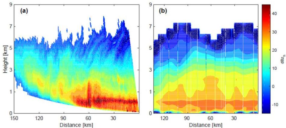
Figure 4 Model-measurement intercomparison of range-height indicator scans of radar reflectivity  $Z_{DH}$  along the 255 degree radial out from CFARR. CAMRa Doppler radar measurements are shown in panel a for the scan taken between 19:22:07 and 19:23:07 UTC, and model are shown from the CTRL simulation at 19:00:00 UTC, both in  $dBZ_h$ .
