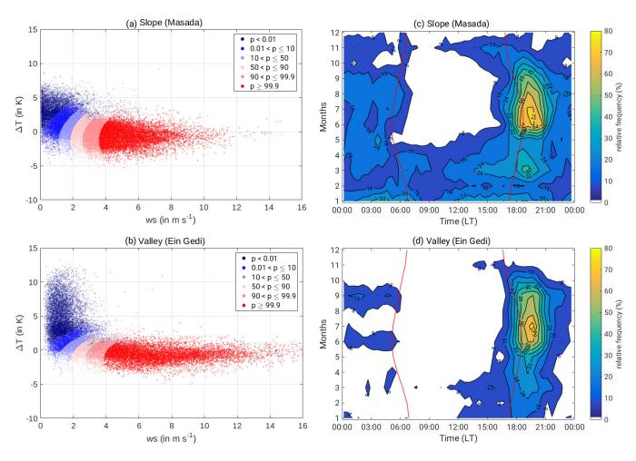
Figure 3. Left: Probability of foehn (colors) for wind velocity and temperature difference ( $\Delta T = T_{crest} - T_{valley}$ ). Right: Relative frequency of foehn occurrence with a detection probability of more than 75 %. Sunrise and Sunset are marked as red lines.
