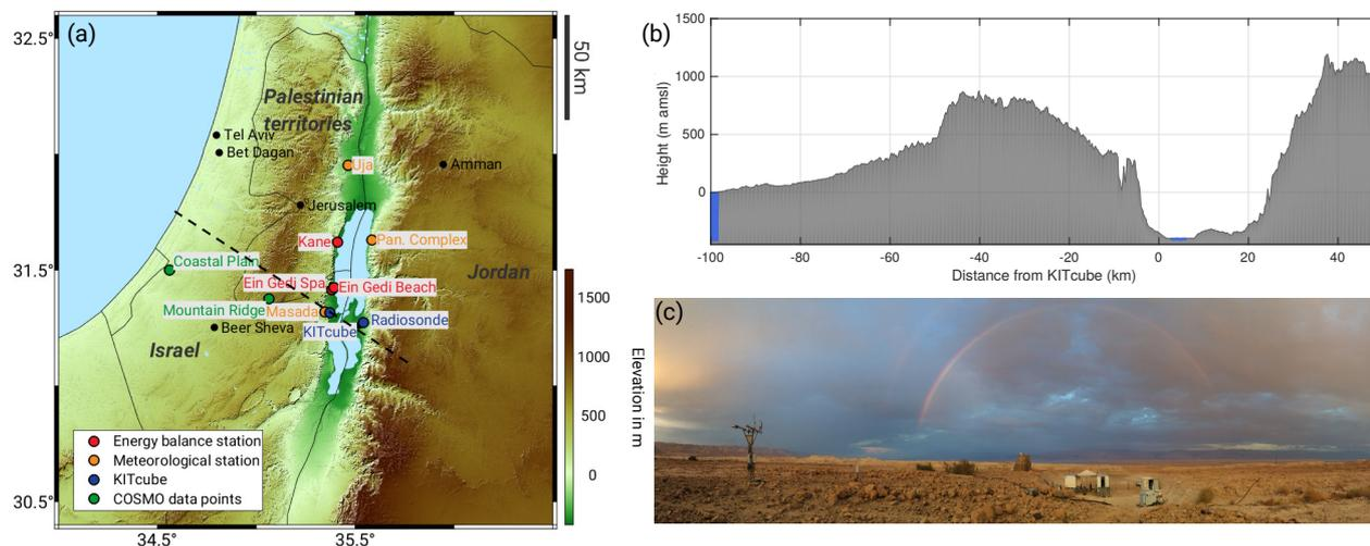
**Figure 1.** Topographic map of the research area with the measurement sites (a). Cross section along the dashed line in (a) is shown in (b), and a picture of the KITcube measurement site near Masada is shown in (c).
