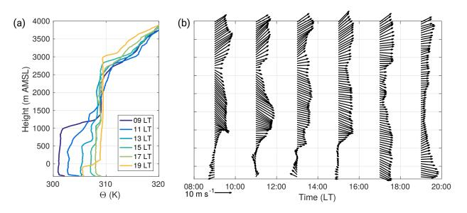
**Figure 8.** Potential temperature (a) and horizontal wind profiles (b), measured with radiosondes in the valley at the KITcube location. Data are shown for 16 August 2014.
