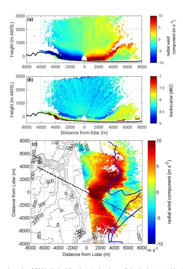
**Figure 10.** RHI scan at an azimuth angle of 299° (dashed line in (c)) showing radial velocity (a) and backscatter (b) on 16 August 2014, 19:36 LT. PPI scan at an elevation angle of 0.2°, shows radial velocity (c) at 19:51 LT. In (a) and (c) blue colours indicate a flow towards the lidar and red colours indicate a flow away from the lidar. The shoreline of the Dead Sea is indicated by a dark blue line in (c).
