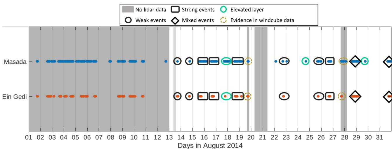
**Figure 4.** Occurrence of foehn in August 2014 at the slope (Masada, blue dots) and in the valley (Ein Gedi, red dots). Shown is the foehn occurrence with a detection probability of more than 75 %. Grey shaded area shows the dates were lidar data were not available.
