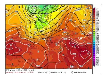
**Figure 7.** Large scale synoptic conditions on 16 August 2014, 15 UTC. Geopotential in gpdm at 500 hPa (black contours), surface pressure in hPa (white contours), relative topography 500/1000 hPa (coloured). Green dot indicates investigation area.
