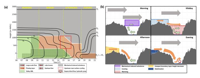
**Figure 12.** Conceptual model describing the different boundary layer processes in the valley on 16 August 2014. The temporal evolution of the different layers and wind systems is given in (a). The wind systems (arrows) and the ongoing processes (shaded areas) leading to the next stage for morning, noon, afternoon, and evening, are shown in (b).
