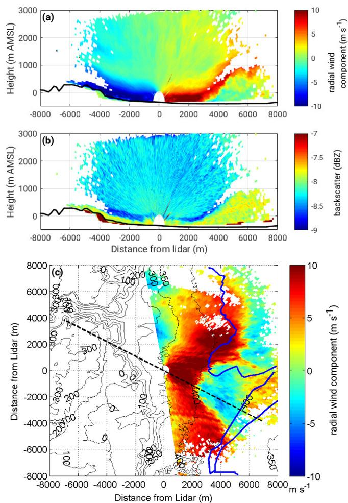
**Figure 10.** RHI scan at an azimuth angle of  $299^\circ$  (dashed line in (c)) showing radial velocity (a) and backscatter (b) on 16 August 2014, 19:36 LT. PPI scan at an elevation angle of  $0.2^\circ$ , shows radial velocity (c) at 19:51 LT. In (a) and (c) blue colours indicate a flow towards the lidar and red colours indicate a flow away from the lidar. The shoreline of the Dead Sea is indicated by a dark blue line in (c).
