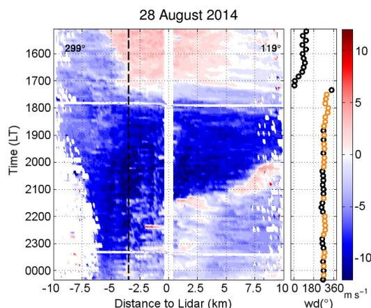
**Figure 6.** Example for a mixed event on 28 August 2014. Hovmoeller diagram of the near-surface radial velocity from lidar RHI scans at an azimuth angle of 299° and 7° elevation west of the lidar and 1.6° east of the lidar. The black dashed line indicates the end of the western slope and the beginning of the valley floor. Wind direction ( $wd$ ) was measured in 40 m agl. Orange points highlight wind directions between 270 and 330°, the main wind direction of the foehn.
