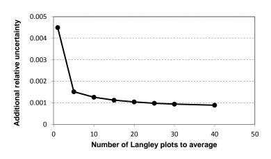
**Figure 6.** Additional uncertainty added to the Langley plot calibration vs. number of Langley plot  $V_0$ 's that are averaged, using GAW-PFR data (500nm) at Mauna Loa (2000-2014).
