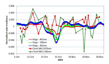
Figure 7. Solar extraterrestrial normalized irradiance as measured by the VIRGO space-based photometer during 2003-2004 at three wavelengths: 402nm (blue), 500nm (green) and 862nm (red).
