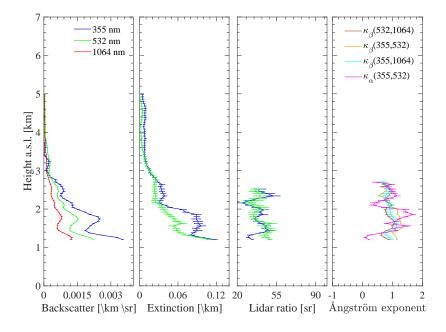
Figure 7. Optical profiles measured at Athens, on 22 May 2014, 20:28–21:28 UTC with a multiwavelength Raman lidar. The error bars correspond to the standard deviation.
