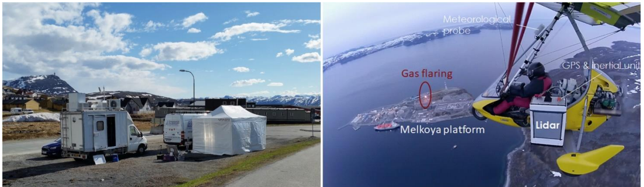
5 Figure 2: Left picture: Mobile atmospheric station (MAS) located near the Hammerfest airport, equipped with the WALI Raman lidar. Right picture: N_2 -Raman lidar LAASURS embedded on a ULA. The ULA is flying over the Melkoya platform where a gas flaring is active.
