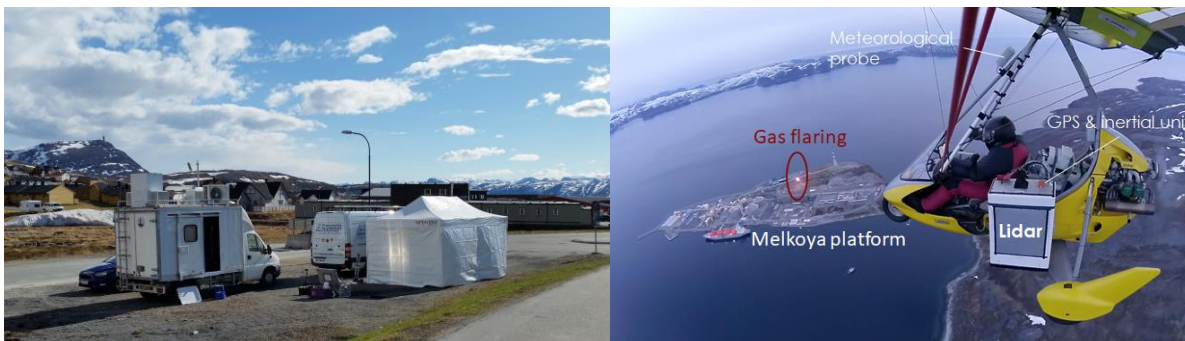
104 Figure 2: Left picture: Mobile atmospheric station (MAS) located near the Hammerfest airport, equipped with the 105 WALI Raman lidar. Right picture: N 2 -Raman lidar LAASURS embedded on a ULA. The ULA is flying over the 106 Melkoya platform where a gas flaring is active.
