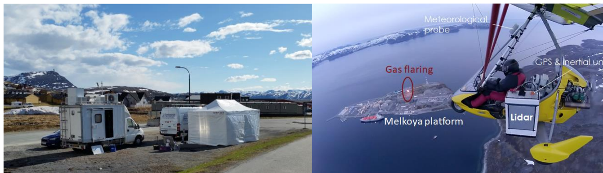
Figure 2: Left picture: Mobile atmospheric station (MAS) located near the Hammerfest airport, equipped with the WALI Raman lidar. Right picture: N 2 -Raman lidar LAASURS embedded on a ULA. The ULA is flying over the Melkoya platform where a gas flaring is active.
