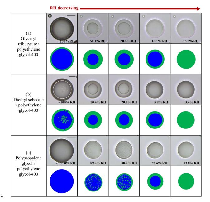
Figure 3. Optical images for particles consisting of two organic species for decreasing RH: (a) glyceryl tributyrate/polyethylene glycol-400, (b) diethyl sebacate/ polyethylene glycol-400, and (c) poly(propylene glycol)/polyethylglycol-400. Illustrations are presented below the images for clarity. Green: organic-rich phase. Blue: water-rich phase. The scale bar is 20 µm.
