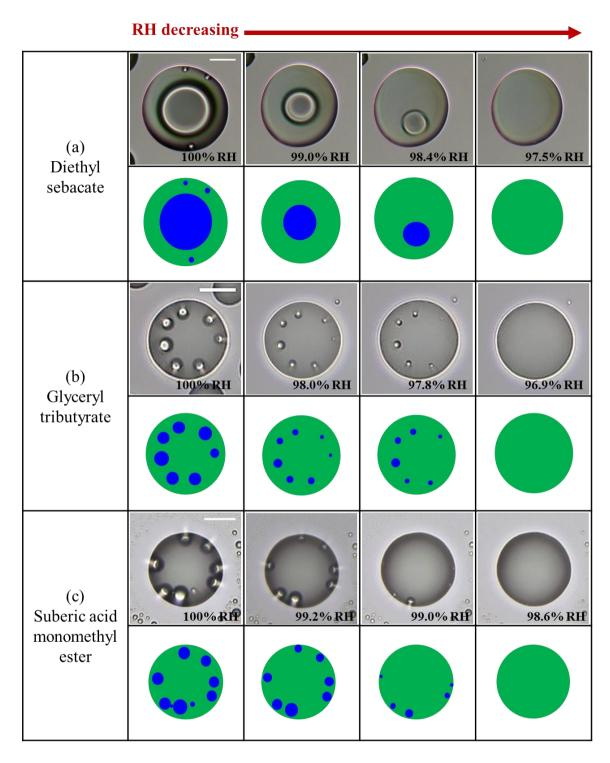
Figure 1. Optical images of single particles consisting of one organic species with decreasing RH: (a) diethyl sebacate particles, (b) glyceryl tributyrate particles, and (c) suberic acid monomethyl ester particles. The "streaks" extending from the inclusions to the edge of the particles in (b) and (c) are an optical effect. Illustrations are presented below the images. Green:
