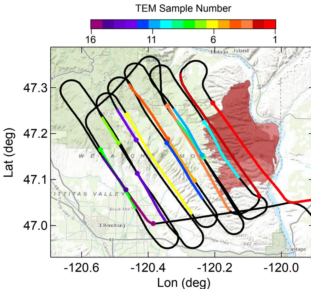
485 **Figure 2.** BBOP G-1 flight track for the Colockum Tarps Fire. Knowing the wind speed and direction, individual transects sample
