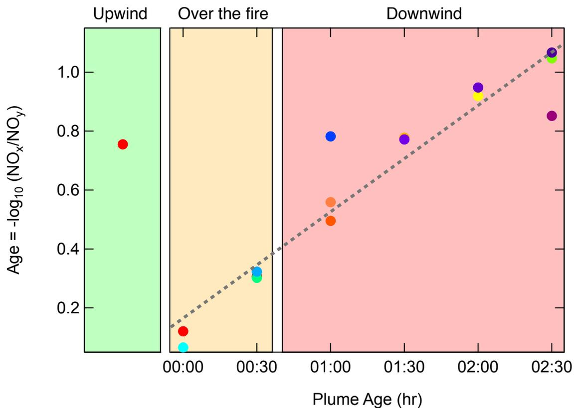
Figure 4 Photochemical age metric,  $-\text{Log}_{10}(\text{NO}_x/\text{NO}_y)$ , as a function of plume age. Clean air background subtracted from  $\text{NO}_x$  and  $\text{NO}_y$ . Grey dotted line is a linear best fit to the dataset. Colors on the plot correspond to those in Figures 2 and 3.
