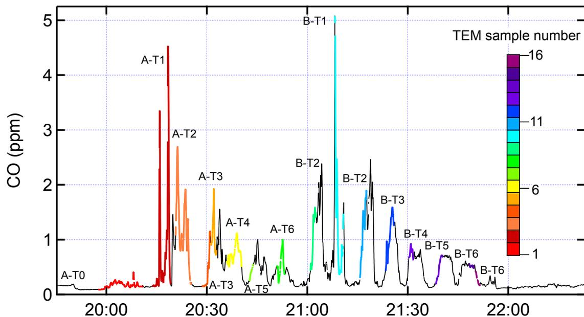
**Figure 3.** Time series for CO, using same color scheme as Figure 2 to label TEM samples. Two sets of transects, called Set A and Set B, cover a similar sampling distance from just upwind of the main fire region (T0) to ~35 km downwind in 6 steps from T1 to T6. Set A encompasses transects A-T1 to A-T6 and Set B transects B-T1 to B-T6. 16 TEM grids were used in this flight.
