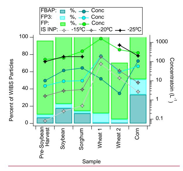
Figure 2. WIBS data showing the concentration (circle markers) and percentage (bars) of three different classes of fluorescent particles (FP, FP3, and FBAP) during the each harvest and one pre-soybean harvest period. The corn WIBS data was collected from the same field but on a different day than the corn IS data. The IS INP concentrations for -15 °C (light grey), -20 °C (dark grey), and -25 °C (black) are shown in diamond markers for non-cyclone samples only.
