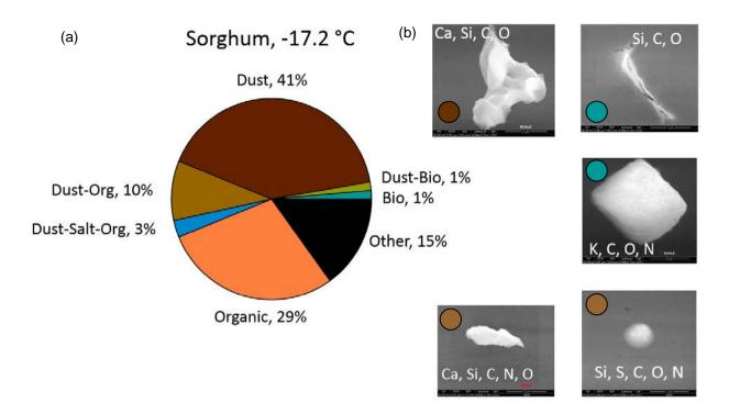
Figure 3. Relative amounts of different particle types collected via impaction and analyzed using SEM-EDX (a) and example SEM images with the corresponding elemental composition measured with EDX shown in white (b). The colored circle in the left corner of the images indicate which chemical class the particles were classified as. These data
