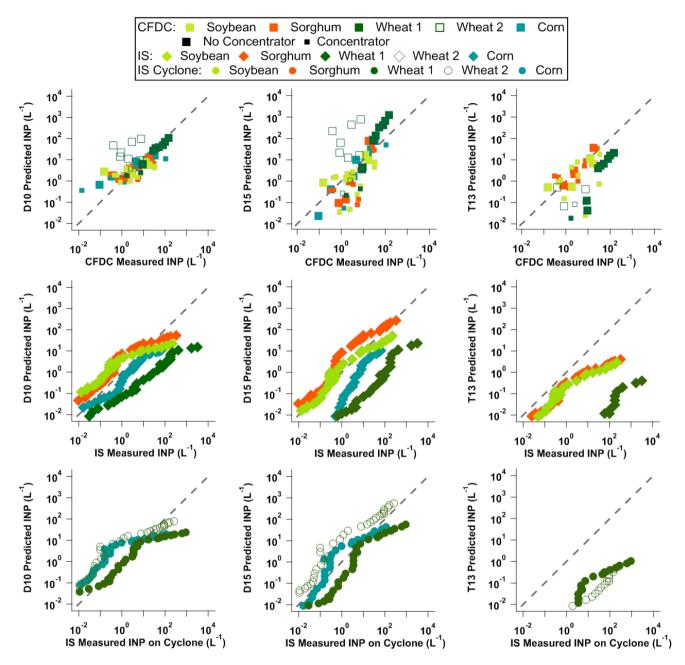
Figure 8. Measured CFDC (top row), IS (middle row), and IS behind a 2.5 µm cyclone (bottom row) INP number concentrations plotted against predicted INP number concentrations using the D10 (left), D15 (middle), and T13 (right)
