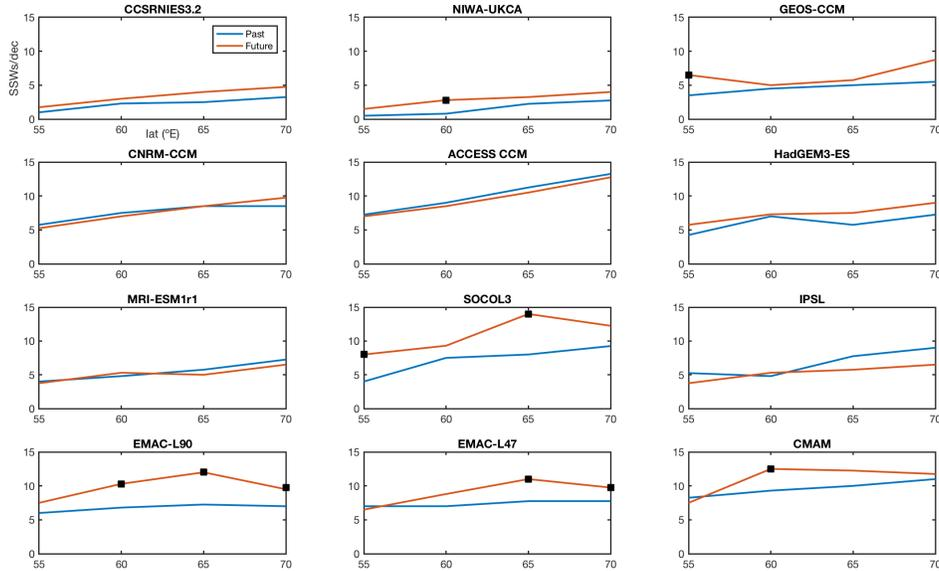
**Figure R2.1.** Mean frequency of sudden stratospheric warmings per decade for the past (blue line) and the future (orange line) in function of the latitude selected for the reversal of the wind. Black squares indicate that future values are statistically significantly different from the past ones at the 95% confidence level.
