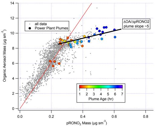
**Figure 6**. Correlation of organic aerosol mass concentration with pRONO<sub>2</sub> mass concentration for the full 2 July flight (grey points and red fit line, fitted slope and thus average OA/pRONO<sub>2</sub> mass ratio of  $\sim$ 30) and for the points during the selected plumes (colored points, colored by plume age, average OA/pRONO<sub>2</sub> mass ratio of  $\sim$ 5).
