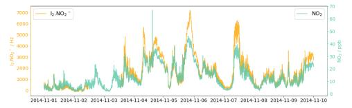
Fig 1.  $NO_2$  measured at the whitworth observatory overlayed with  $I_2$ - $NO_2$  measured on the ToF-CIMS.  $NO_2$  is overestimated by the ToF-CIMS at high concentrations. This is potentially due to the degredation of NOy species in the IMR.
