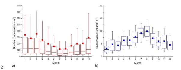
1. Monthly average variation of (a) nucleation mode particle number concentration and (b) sulfuric acid condensational sink (*CS*) at Finokalia station over the period June 2008-June 2018. Whiskers represent 10th and 90th percentiles, box edges are 75th and 25th percentiles, the line in the box is the median, the solid square is the mean.
