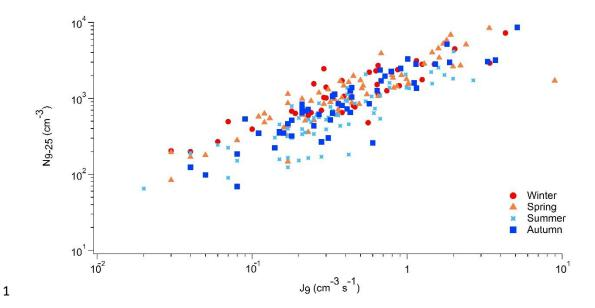
7. Scatter plot of the number concentration of nucleation mode particles ( $N_{9-25}$ ) (hourly maximum value during the event) versus formation rates of 9-nm particles ( $J_9$ ) at Finokalia, for events when  $J_9$  could be calculated with a good level of confidence (Class I events).
