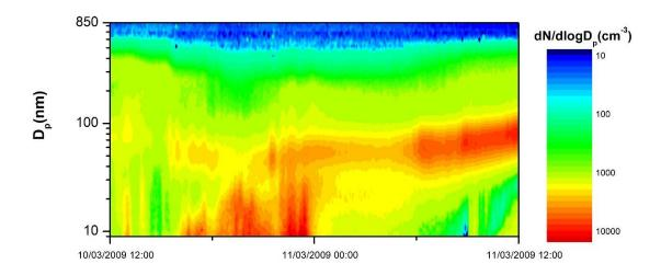
3. Example of appearance of nucleation mode particles during several hours as observed during the night of 10 to 11/03/2009 (time in UTC+2).
