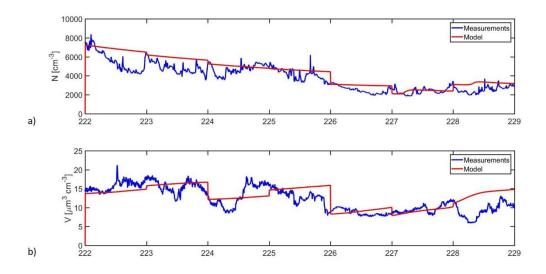
12. Simulations with the MALTE box with the adjusted parameters for the sub-tropical environment for the "non-event" week that no NPF was observed at Finokalia. Measured and modelled (a) total number concentration and (b) total volume concentration for the same period. The x-axis in both figures is Julian day of 2012.
