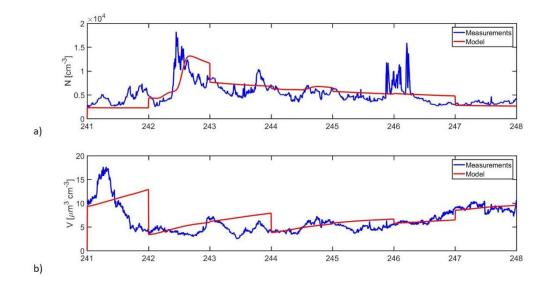
11. Simulations with the MALTE box with the adjusted parameters for the sub-tropical environment for the "event week" that NPF events were observed at Finokalia. Measured and modelled (a) total number concentration and (b) total volume concentration for the same period. The x-axis in both figures is Julian day of 2012.
