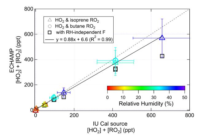
Figure 2. Results of the calibration comparison in which ECHAMP measured the total peroxy radical concentration in the output of the IU calibration source. The error bars indicate  $2\sigma$  uncertainties of the ECHAMP measurements and IU calibration source, adjusted for the fact that the IU actinometry was based on the ECHAMP NO<sub>2</sub> calibration. The slope of the dotted line is unity.
