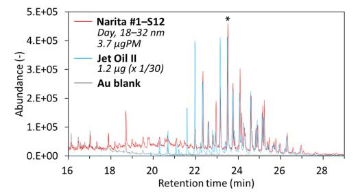
Figure 3: Mass chromatograms (m/z 85) of a nanoparticle sample collected during the daytime (sample #1, February 9–13, 2018; S12, diameter: 18–32 nm) at the Narita International Airport, Jet Oil II, and Au-foil blank. The mass spectra of the peaks at 23.51 min of Narita #1–S12 sample and Jet Oil II with an asterisk are shown in Fig. 4.
