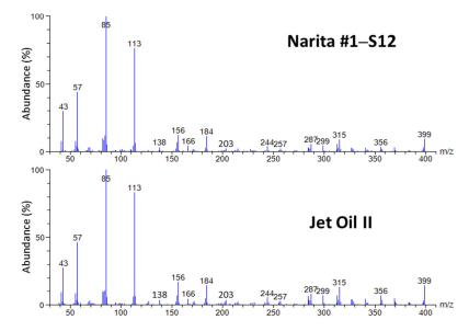
Figure 4: Mass spectra of a nanoparticle sample collected during the daytime at the Narita International Airport (sample #1, February 9-13, 2018; S12, diameter: 18-32 nm) and Jet Oil II at 23.51 min of the TD-GC/MS chromatograms. The chromatographic peaks are indicated in Fig. 3. The instrument background spectrum was subtracted for the Narita #1-S12 sample.
