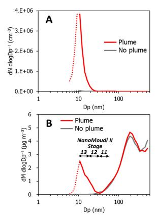
Figure 1: Size distributions of particle concentrations with and without aircraft exhaust plumes. (A) Particle number concentrations. (B) Estimated particle mass concentrations. The averaging times are approximately 20 s for both events. The measurement periods were 11:43:42–11:44:01 on February 15, 2018 and 11:43:11–11:43:30 on February 15, 2018 for the "plume" and "no plume" events, respectively.
